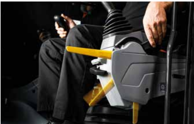
The pilot shutoff lever offers enhanced safety in the cab.
