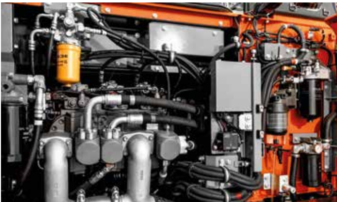
New layout provides convenient access to all filters.
