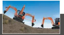
Higher gradeability and work capability Thanks to the high tractive effort and strong swing torque, the DX85R-3 offer excellent capability for working on slopes.
