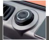
RPM dial / Auto idle Thanks to the electronic control, the optimal engine rpm can be set per workload. The auto idle function applied as standard helps fuel efficiency
