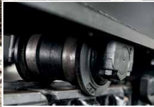
Strengthened bushing material improves wear resistance.
