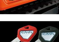
The red programming key programmes the individual keys. The individual black keys start the engine.
