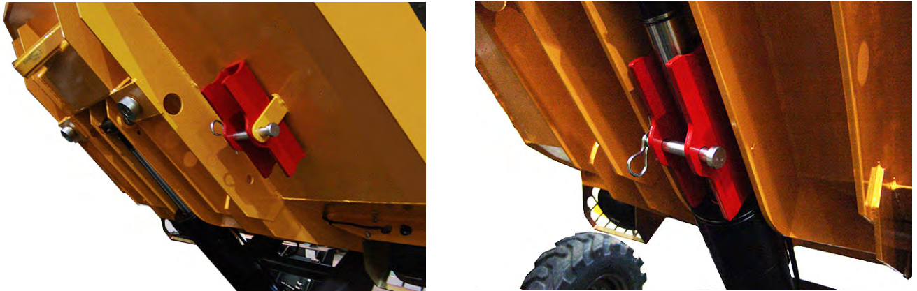
Figure 9.3 - Skip Prop - Swing Skip Machines - stored and in position
