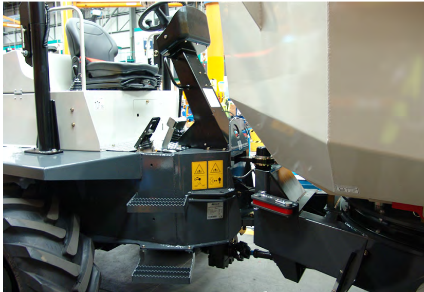
Figure 4.2 - Machine access - steps
