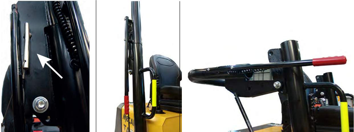
Figure 7.1. - Linch pin, handle and ROPS work position
